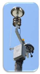
Thor Guard reads the activity of the electrostatic field in the atmosphere and predicts the probability of a lighting strike within a predetermined area. When the system detects the possibility of lightning, a loud siren is produced by a cluster of horns
