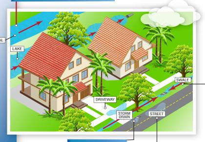
Storm drains draw water into an underground drainage pipe that moves it to a lake or canal.
