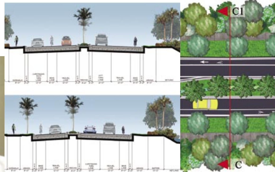
Left top: Extension of the right-turn lane between Vista Park Boulevard and Isles of Weston Avenue, section view; Provisions between South Post Road and Park Ridge Street plan view. Left bottom: Provision of Bike Lanes across from Manatee Bay Elementary, section view.
