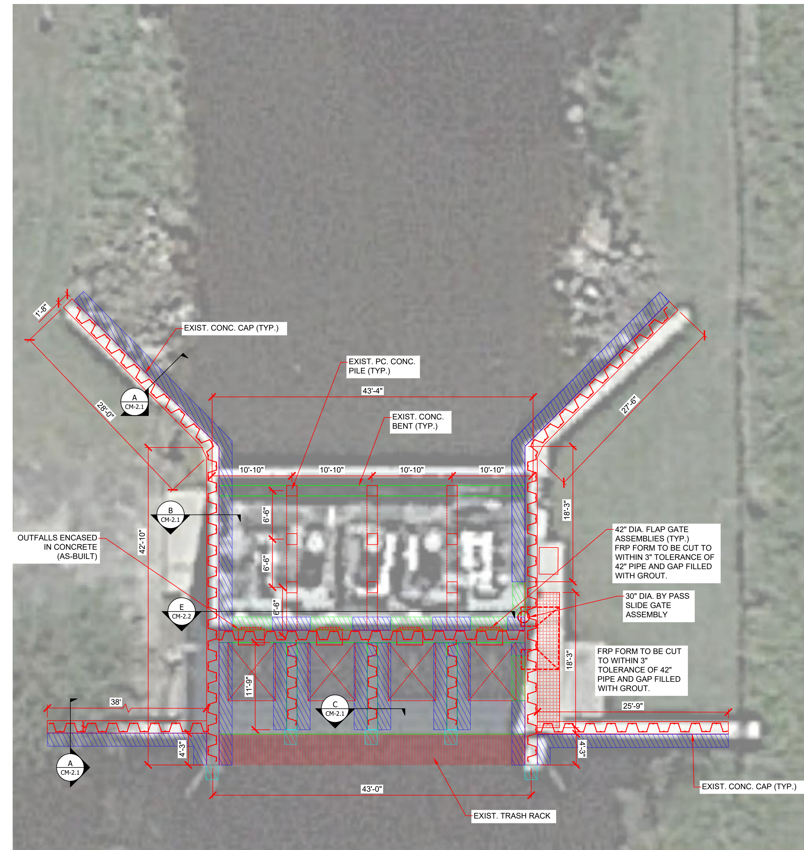
PUMP STATION #2 BULKHEAD ENCAPSULATION PLAN
