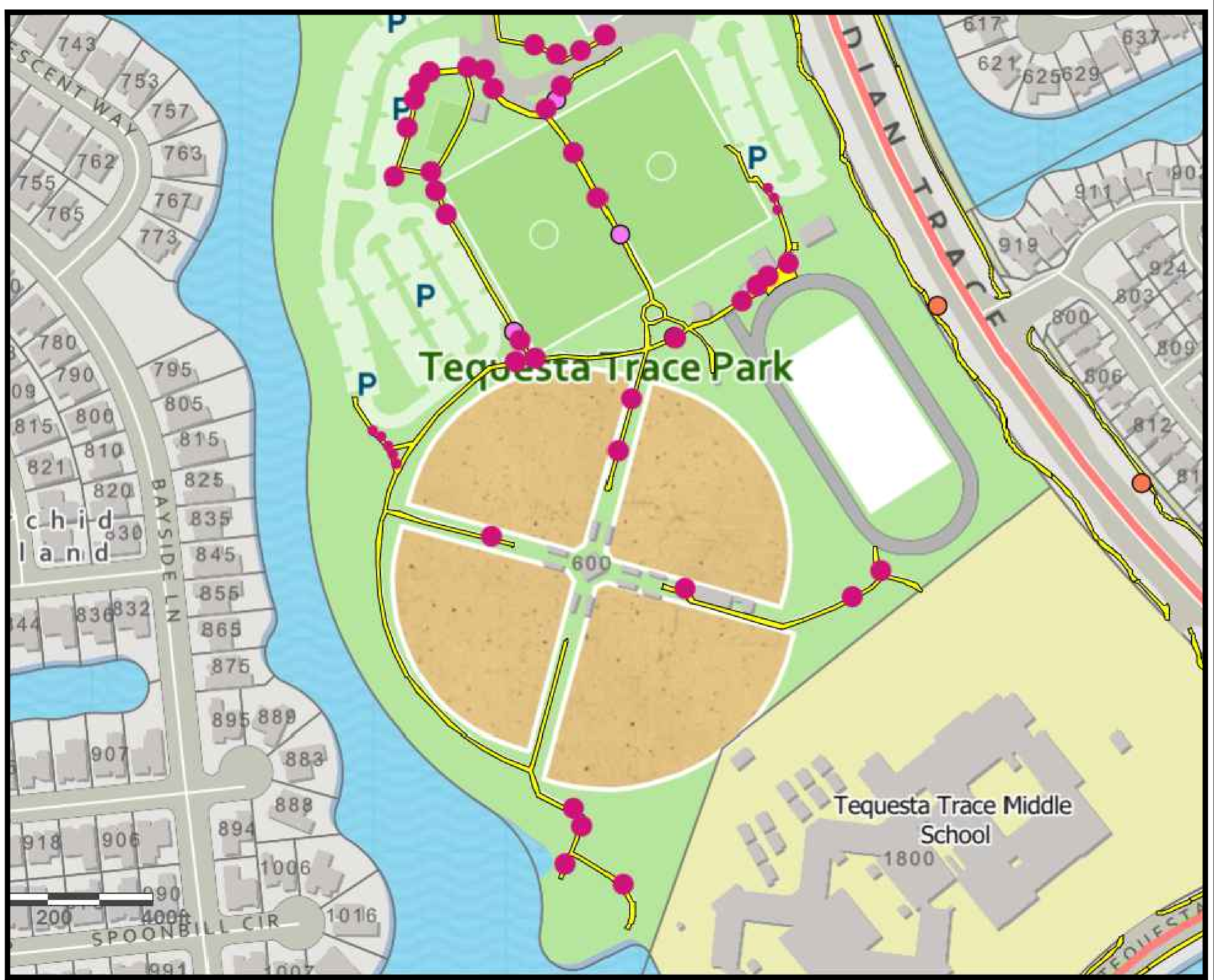
LOCATIONS OF DAMAGED SIDEWALKS AT TEQUESTA TRACE PARK (COORDINATE WITH THE CITY FOR LIMITS PRIOR TO REMOVAL)
